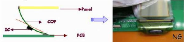
12.6 Use both thumbs to insert COF into the connector when assembling the panel. See the photo on the far right below for correct insertion of the film into the connector (one-handed insertion exerts uneven force on the film and could cause its breakage, photo on the left)
